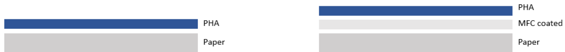
Figure 3. Schematic of PHA applied on paper substrate, with or without MFC pre-coating.
