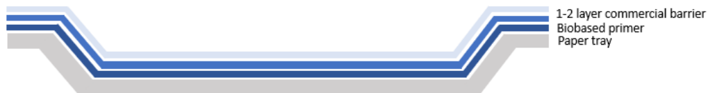
Figure 18: Schematic of single or multilayer spray-coated cellulose tray substrate with biobased primer
