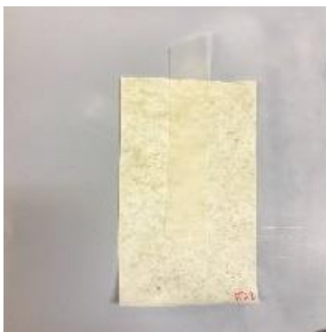
Figure 10. Example of the placement of a 1.5 cm film strip on a 6 x 12 cm PHBV coated paper prior to lamination in hot-press.
