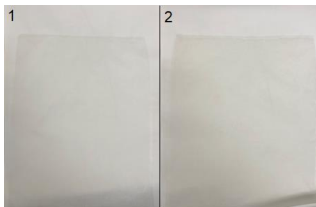
Figure 35. Pictures of carnauba wax with chitosan formulation coated on kraft paper, 1 and 2 layers.
