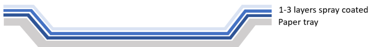
Figure 38: Schematic of single or multilayer spray-coated cellulosic tray substrate
