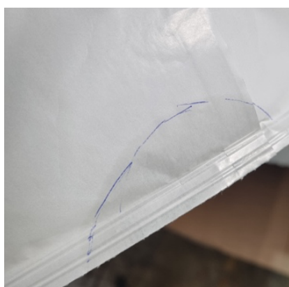
Figure 25 : Grease leakage on the sealing area observed after conditioning chips in paper-based flexible packaging
